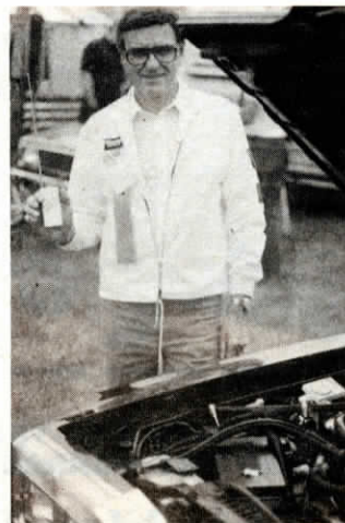
Transmitter activates pump and heater controls, circulating coolant to warm up both engine and inside of car.
