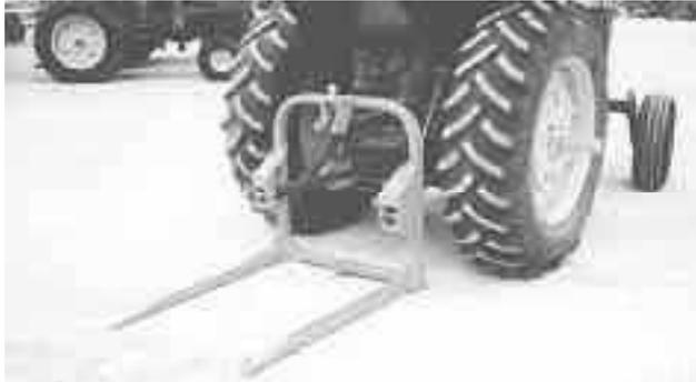
Hitch lowers flat to ground so no jack is needed to raise implement tongues. Hitch tongue adjusts from center to either side and allows use of pto without interference.
