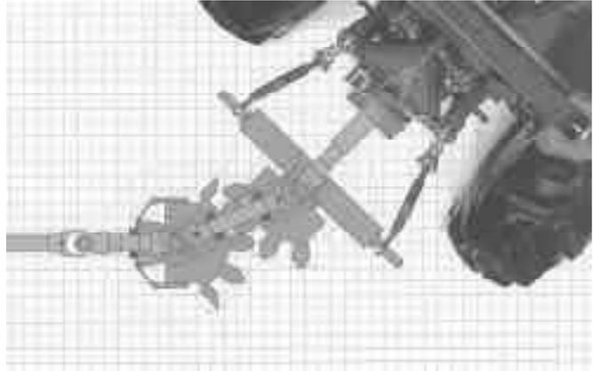
Constant velocity hitch hooks up to lift arms on tractor's 3-pt. hitch. A pair of cogged steel wheels connect hitch to implement drawbar.
