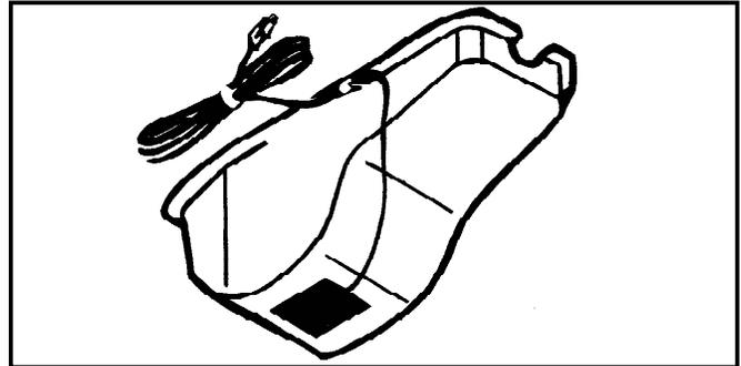
Preheater pad adheres to bottom of oil pan. Can be used on any pan or even on oil barrels.
