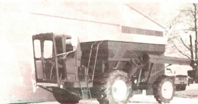
Wammes used the engine, drive train, cab, rear axle and fuel tank from an old Ford combine to build the grain buggy.
