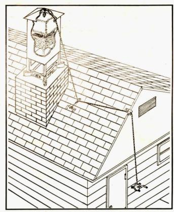
"Remote controlled" brush cleans chimney in less than a minute.
