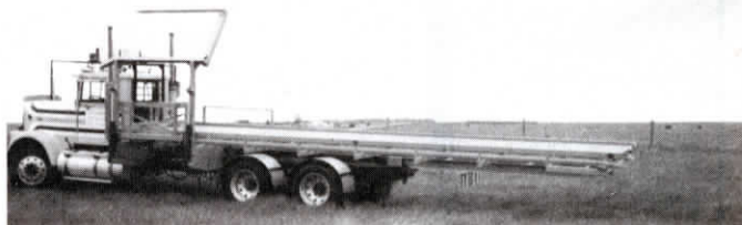
Special-built bale deck is designed to mount on a semi tractor. A smaller deck for 3 to 5-ton trucks is also available.
