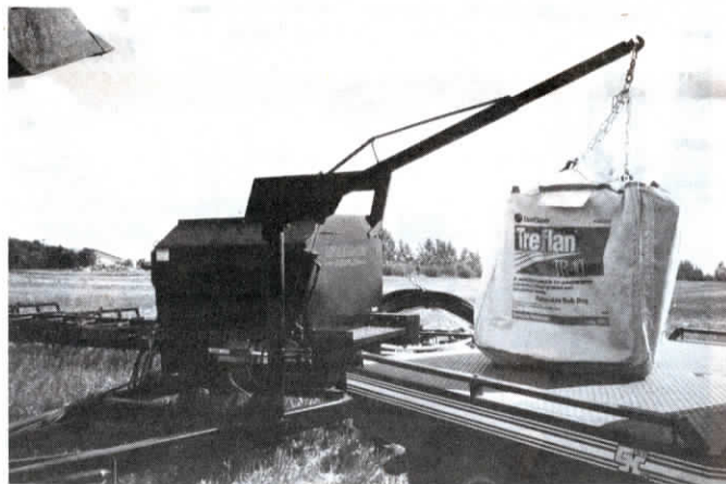
Bag lifter boom clamps onto frame of implement to handle bulk bags.
