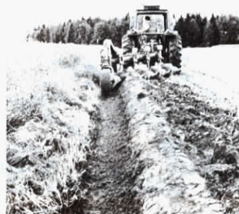
Photo on right shows plow working next to ditch bank. Left photo shows how furrow wheel and hub of rearmost disk determine how near to obstructions plow can operate.
