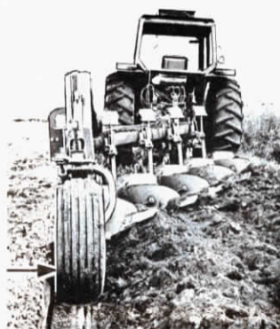
Photo on right shows plow working next to ditch bank. Left photo shows how furrow wheel and hub of rearmost disk determine how near to obstructions plow can operate.
