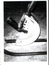
pipe and pulls backward. When the handle reaches the ground, it has made a 45° bend in the tubing. Then he slips the handle out and slides it into the pipe's other open end to complete the 90° bend.
