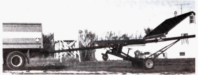
Front drive wheel lifts for down the road towing.
