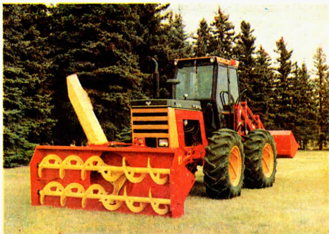
One equipment combo made possible by new tractor is this front snowblower and rear bucket match-up.
