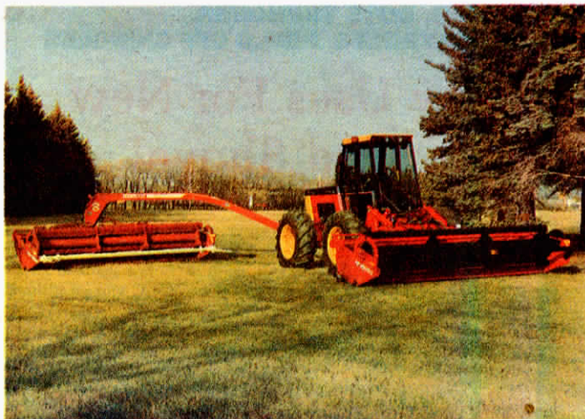
Outfitted with two 14-ft. auger headers, tractor cuts a 28-ft. swath. Reversible controls and hydrostatic drive make rear operation no different than forward travel.
