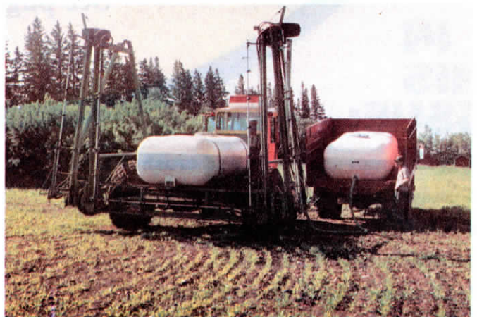
Boom folds hydraulically for transport. Two large wheels support each wing.
