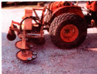
Edges of cutting discs are covered with rubber and small roller wheels on leading edges help roll trim arm around trees and other obstacles. (Photo shows unit mounted on side of rear mower.)
