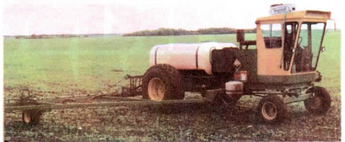
Meyer put truck suspension under the front-end of 72-ft. combine sprayer so that it "rides as good as a pickup" in the field.
