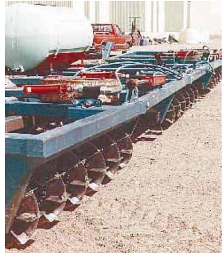
The 32-ft. unit is equipped with two rows of cutting wheels that Fuesz built by mounting pairs of 3 1/2-in. wide steel knives on 18 1/2-in. dia. cutting wheels.
