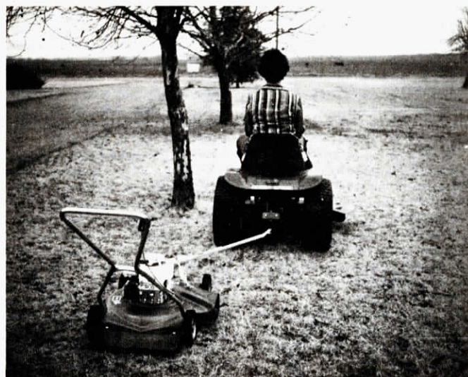
Rollers built into tow hitch automatically roll trailing mower, or mowers, around trees and other obstacles.
