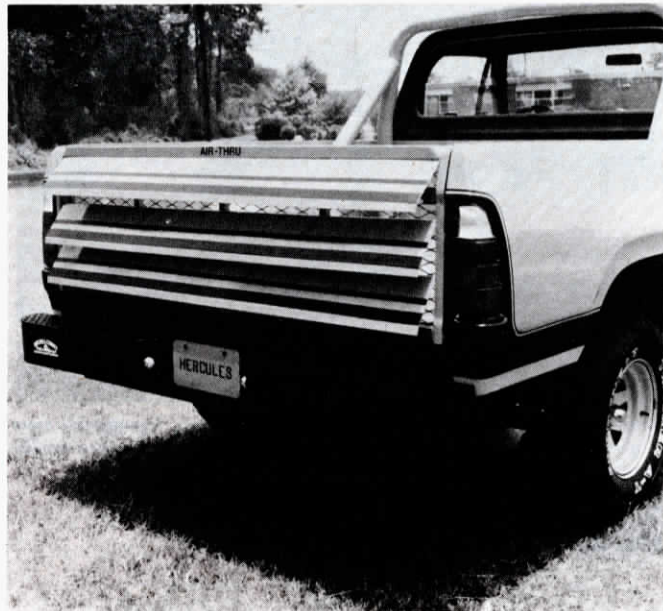
"Louvered" tailgate saves up to 15% on pickup gas bills by allowing air to flow through at speeds of 25 mph or more.
