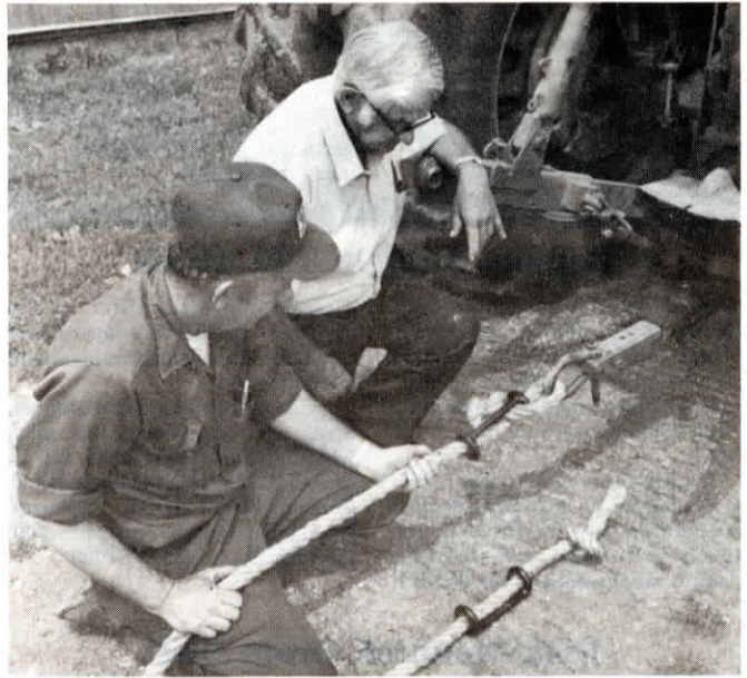
Rope is threaded through both loops of Happy Hooker, through the clevis, and back through the Happy Hooker. Then the end is tied in a knot.
