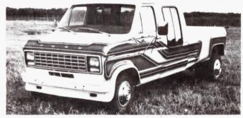
L & D Manufacturing in Sturgis, Mich., makes this truck-van combo. The Dodge hybrid is equipped with a 460 cu. in. engine, no longer available in pickups.
