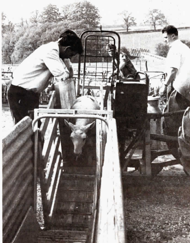
Sheep are herded up the trimmer's ramp and over the abrasive belts. A triangular hoof divider keeps their feet on track and in position.
