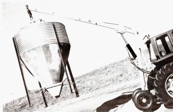
New hydraulic boom is shown extended to its full length of 15 ft. Lifts up to 2,500 lbs. at this fully-extended point.
