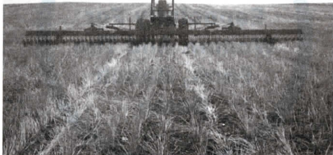
Heintzman equipped two 41-ft. Yetter minimum-till rotary hoes with his kit to convert them into no-till rotaries that walk right through heavy "bumper crop" residues.
