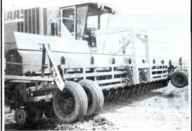
Kit includes extension arms which reposition wheels for greater residue and rock clearance, and new-style mounting bracket with built-in sealed bearing and dust protector.
