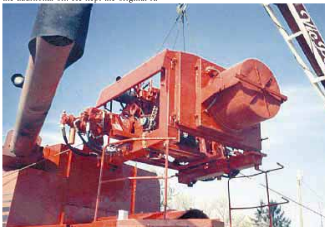
Moore used 7-in. sq. steel tubing to build new subframe for engine that also is a two-part oil reservoir. He also installed a hydraulic pump-drive on each end of engine.
