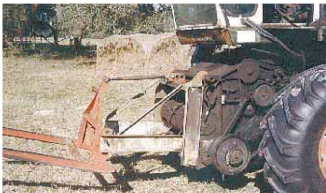
He used channel iron and header hooks off an old corn head to make a 3-pt. frame that fits to feederhouse. A set of bale forks mounts on frame.
