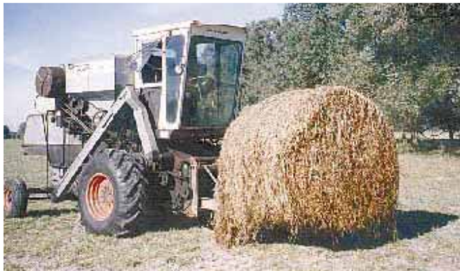
Nelson fitted combine with a quick tach mounting arm. He still uses the combine for harvest.
