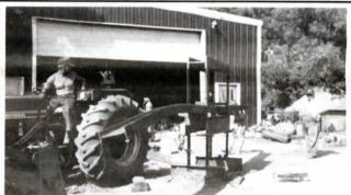
Heinze built this press to straighten 12-in. wide steel I-beams used on his machine shed. He uses an IH 784 tractor to power the press's 5-in. hydraulic cylinder.
