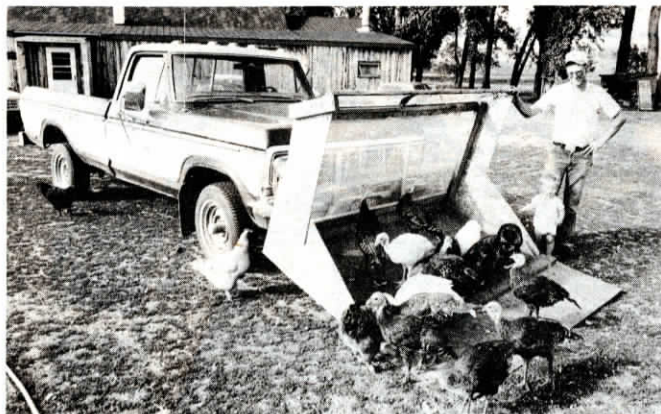
Ponzer has caught up to 17 gal. of hoppers in one 30 min. run with his 6-ft. wide catcher.
