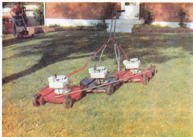
Bud Hoekstra says he cut an unpleasant job down to size by linking three lawn mowers together.
