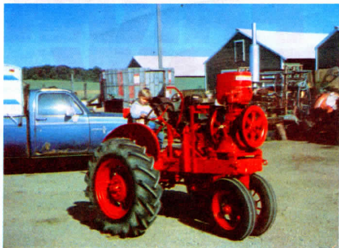
Hoppe shortened up this Allis Chalmers WC and powers it with a 3-hp. Ideal upright antique gas engine, which chain-drives the tractor's transmission.
