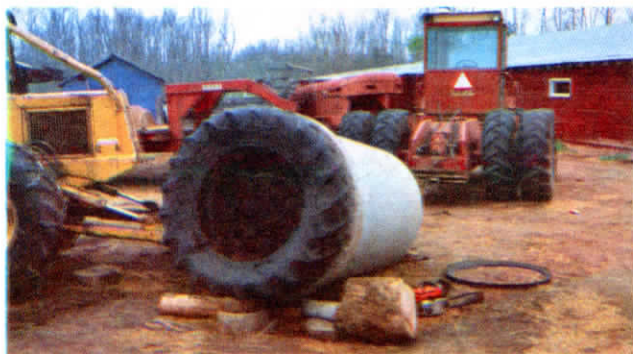
You can use different size culverts to turn different size tires, says Westerlund.
