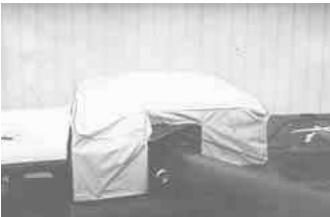
New hopper cover can even be used while harvesting since it doesn't interfere with combine unloading auger.
