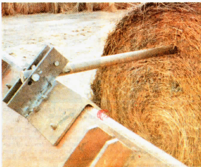
Above photo: Angle iron spreads weight along top of bucket to avoid bending. Spear (7 ft. long, 2 in. in dia.) removes by pulling one pin.
