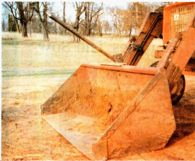
Angled spear is out of way and can be left on when using the bucket for loading snow, silage or manure.
