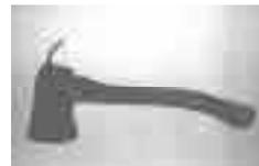
I use a small ax to cut strings on hay bales. I weld a hook on back to break the bales apart. I can also use the hook as a "pickaroon" to handle logs when sawing wood. Very handy. (**Walt Austin, 19544 Johnson Creek Rd. S.E., Tenino, Wash. 98589 ph 206 264-5491**)
