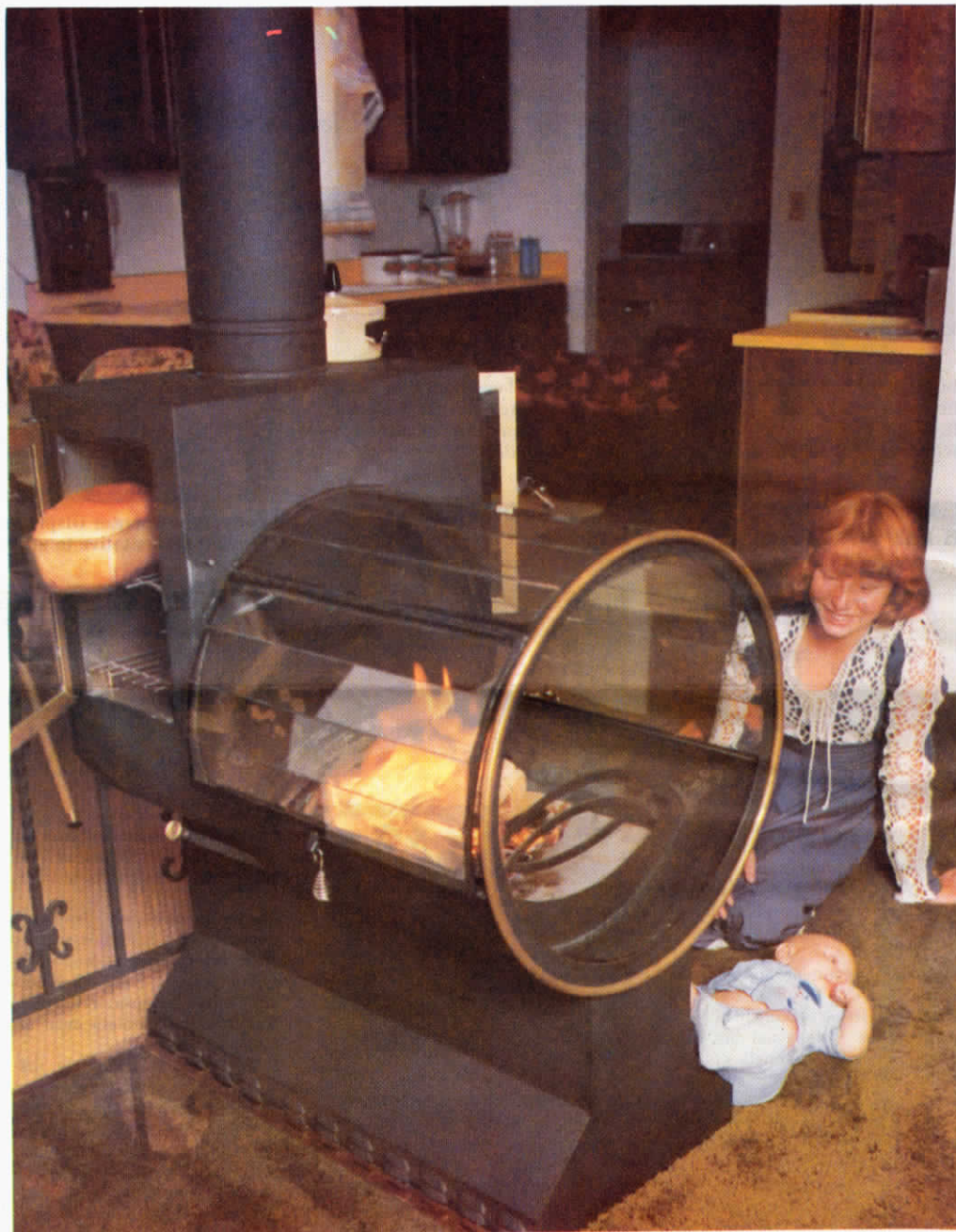
Glassed-in firebox allows fire to fill the room with light. Exterior of firebox gets hot and will burn fingers if touched, but bottom pedestal remains relatively cool. Freestanding unit can be installed directly on a carpet or bare floor.
