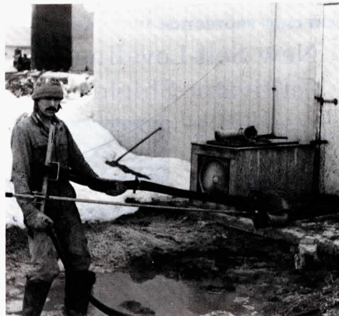
New Farmstar Pit Pal, left, chops, agitates and unloads pits or lagoons. It slips through a 20-in. opening.
