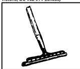
You can make a quick and handy squeegee for cleaning any concrete floor. Just slit a piece of rubber garden hose and slip a garden rake into the slit as shown.
