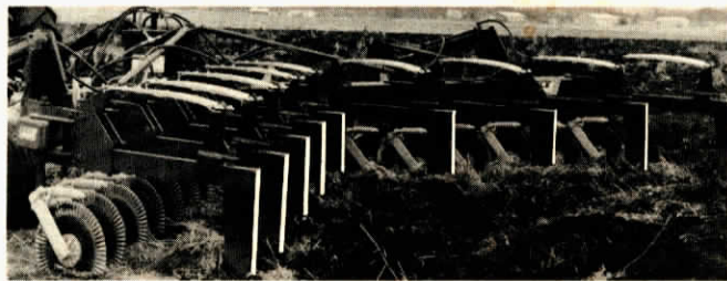
Width of v-shaped subsoiler adapts to field conditions.
