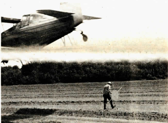
Each spoke is spaced 3 ft. apart, so you can precisely "walk off" distances across fields.
