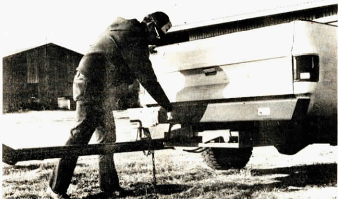
The air bumper features an optional telescoping pickup hitch that uses heavy latches instead of wear-prone springs or catch pins.
