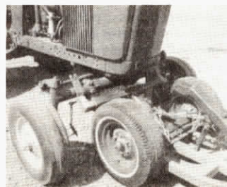
Tractor front axle is cradled in cart's lifting arm, then driven forward to raise front wheels off ground for transport.
