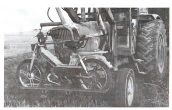
I farm in France and have 50 pieces of land scattered out. Some are several miles from home. It's always a problem at harvest to move all the machinery around. I solved the problem by using steel tubing to make a Moped carrier that mounts on front of all of
