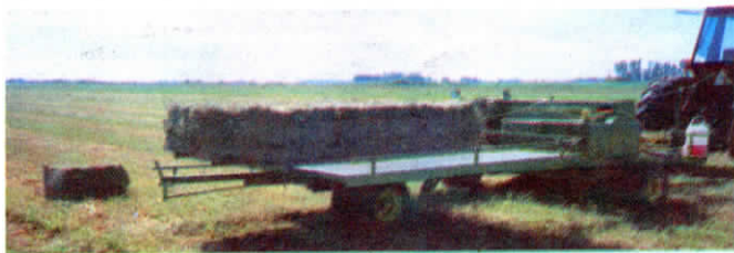
Accumulator attaches to back of baler and rides on single castor fitted with dual wheels. Bales exit bale chamber onto small table that holds three bales end-to-end.
