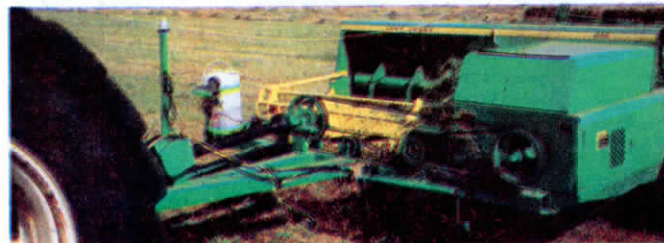
Richards modified baler to run directly behind tractor with pto-driven belt drive.
