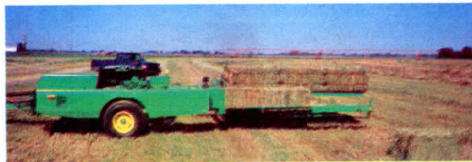
Bales are rotated 1/4 turn onto their sides as they're lifted onto table. Each row pushes previous row over until there are 7 rows.
