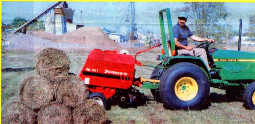
Pto-powered, fixed chamber mini baler mounts on tractor 3-pt. Requires a minimum 18-hp. tractor.
