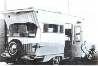
Sterling Weber built the "Cozy Cruiser" into the trunk and rear seat of his 1957 Chrysler Imperial 4-door sedan. Aluminum panels are fastened to a wooden framework that's bolted to an angle iron frame welded along the inside of the car. The car's original rear window, placed upside down, serves as the motorhome's rear window.
