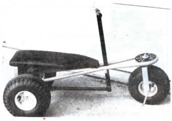
Pushing or pulling on the handle turns a crank mounted between the rear wheels.
