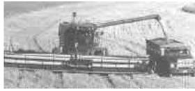
FARM SHOW readers might be interested in my flexible spout extension for combine unloading augers. Problem is that when you're unloading into a truck or wagon onthe-go on a windy day you can lose a lot of grain because of the distance it has to drop from the end of the auger to the truck or wagon box. My spout extension remedies that problem by channeling grain into a smaller drop pattern. The one pictured, on
