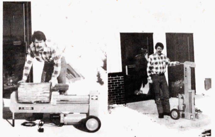
Danuser 110V electric splitter stands vertically for out of the way storage when not in use.
