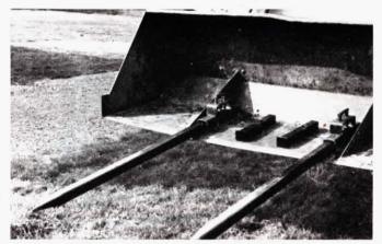
"Easy Tach" forks slip into permanent mounting plates on loader bucket.
