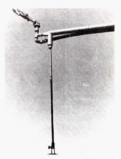
The 4 ft. "Flusher" screws into the conventional sand trap. A steel plate, below, deflects sand and water as it shoots out of the center pivot, preventing damage to crops below.
