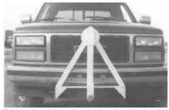
Hitch bolts to frame of pickup and has telescoping tow bar with maximum draw weight of 6,000 lbs. When not used for towing, it folds up flat against front of pickup.
