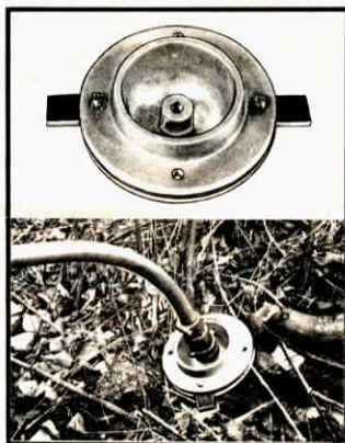
Brush cutter mounts with one bolt. Blades swing freely on mounting studs.
