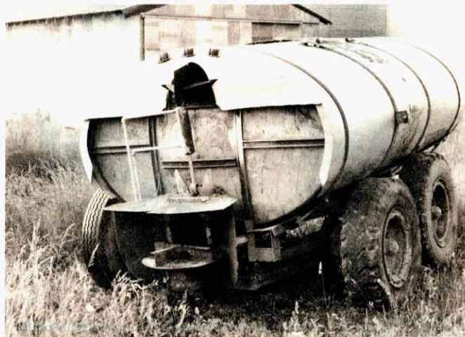
Manure flows out 12 in. hole in rear and onto a fan-type, pto-driven spreader made of stainless steel.
