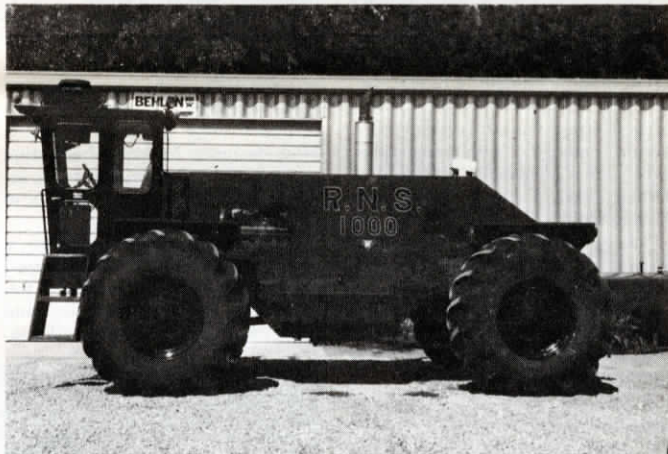
Cab on new RNS tractor sits forward for clear, unobstructed view. Hood raises automatically for easy access to engine, transmission and other parts.
