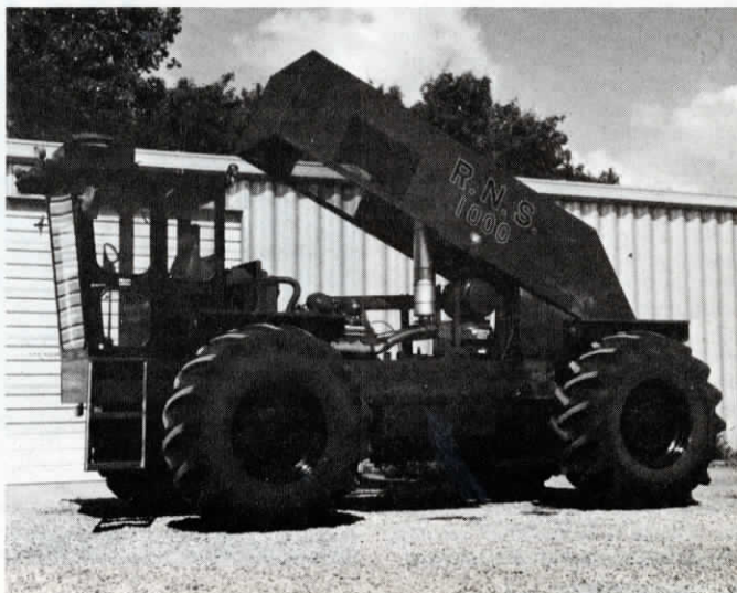
Cab on new RNS tractor sits forward for clear, unobstructed view. Hood raises automatically for easy access to engine, transmission and other parts.
