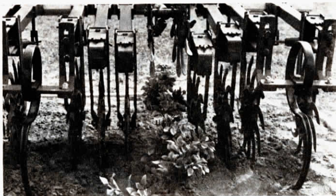
The Hoe-N-Till's row gang units (raised above the row) weed crops like a rotary hoe. Spider wheels and Danish tines (between rows) dig deeper for more aggressive cultivation.
