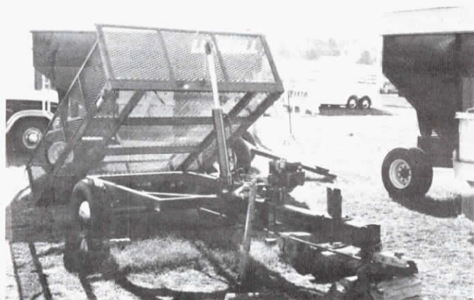
The splitter, mounted on the trailer's tongue, handles logs up to 36-in. in length.
