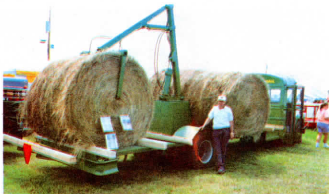
Mid-mounted boom picks up big round bales on either side of bus.
