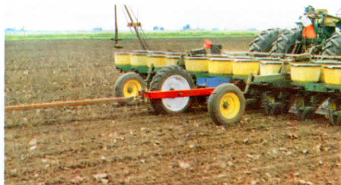
Hitch on back of add-on wheel tows a flatbed wagon loaded with seed and tools. "We can plant corn without having to use another support vehicle," says Wessels.
