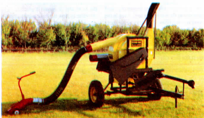
Home-built "Econo-Vac" uses a fan to move grain instead of a positive displacement pump and eliminates the need for an air lock, greatly reducing the cost of machine.
