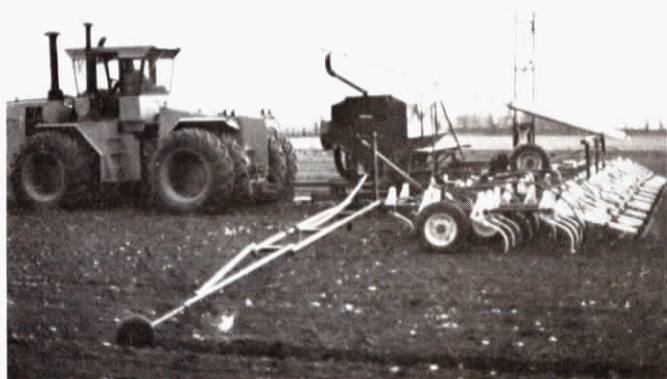
New Wil-Rich air Seeder-Cultivator will handle most types of seed and granulated chemicals, fertilizer.
