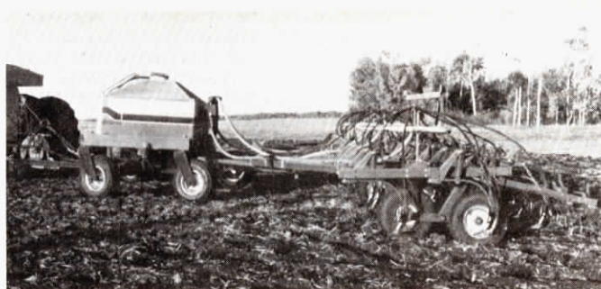
The Super Seeder is available with a 125 bu. grain tank, or with a combination grain tank (65 bu.) and liquid fertilizer tank (300 gal.).
