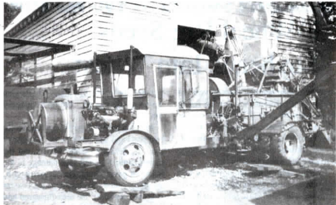
Self-propelled sheller mounts on a GMC truck frame and is powered by a 327 cu. in. engine. Schroeder switches driveshafts when changing from road travel to shelling.
