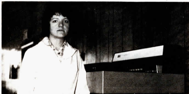
Roxann Caswell, Mid States Lab Technician, operates Scintillation Counter which "reads" milk sample to determine if cow is pregnant.
