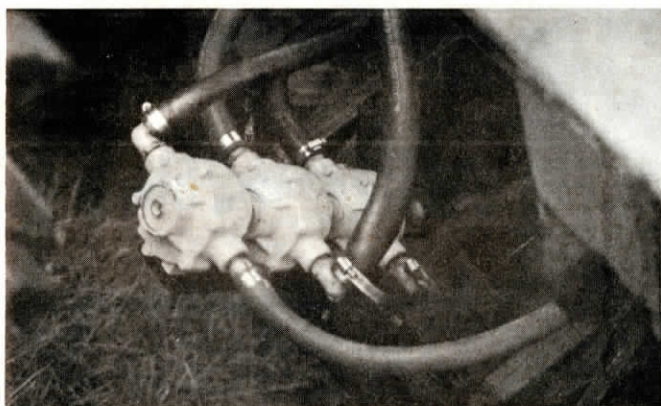
The three in-line pumps connect to hoses from three separate chemical tanks.
