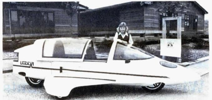
Powered by a 450 cc. Honda motorcycle engine, the car is equipped with a two speed automatic transmission.
