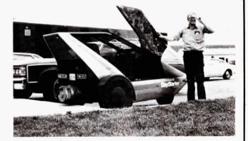
2,220 lbs. is in the 13 batteries, which ride only 8 in. off the ground. The car's Volkswagen transmission has four speeds forward and one in reverse. Windows are plexiglass and the body aluminum. The car's electric motor was obtained from a truck company that had used it in an experimental electric
